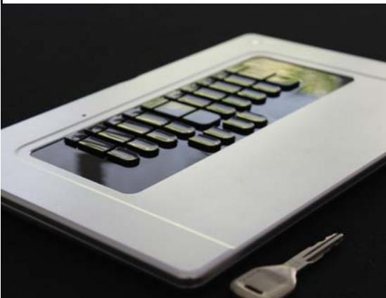
Those features are complemented by the unique ability to adjust each individual key's sensitivity by means of a simple graphical user interface in a computer program.
